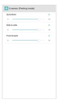
The G-sensor measures the movement of your vehicle through 3 axes – up and down, side to side, and front and back. When the G-sensor detects significant or sudden movement (such as an impact or collision) it will trigger an event recording. You can adjust the sensitivity so minor incidents and bumps don't trigger an event recording. To turn off event recordings by impact detection set the G-sensor sensitivity to off.
